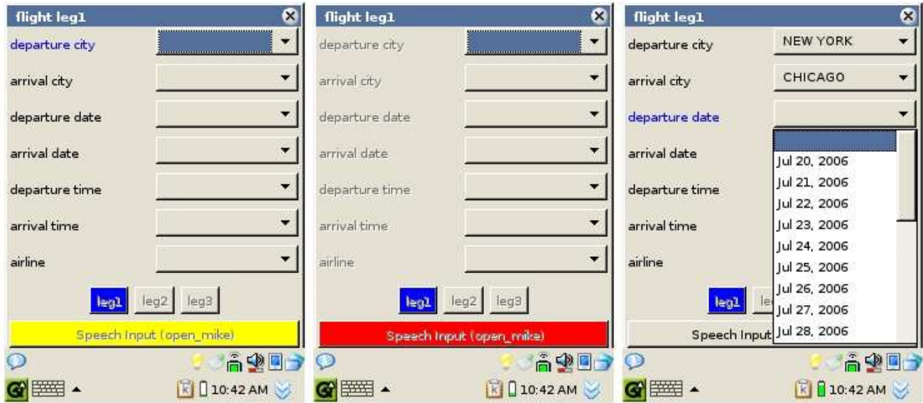
Figure 1: “Modality-Selection” interaction mode examples on the PDA. System is in “Open-Mike” mode in the first frame (speech button is yellow indicating waiting for input), receives user input “From New York to Chicago” during the second frame (speech button is red showing activity) and switches to “Click-To-Talk” mode in the third frame. The speech/pen input default mode is selected by the system in the first/third frame, respectively, due to the large/small number of options in the combo-box.
