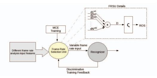
Fig. 1. Variable frame rate speech recognition system
