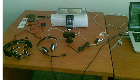
Fig. 2. Evaluation setting. Depicted counter clockwise is the iPhone device, the GSR apparatus (arduino and breadboard), the Emotiv device, the audio headset and the PlayStation Eye camera.
