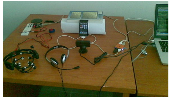
Figure 1. Evaluation setting used for the multimodal iPhone application. Depicted counter clockwise is the iPhone device, the GSR apparatus the Emotiv device, the audio headset and the PlayStation Eye camera.
